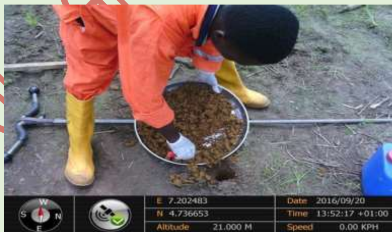
Back filling of Auger Hole
