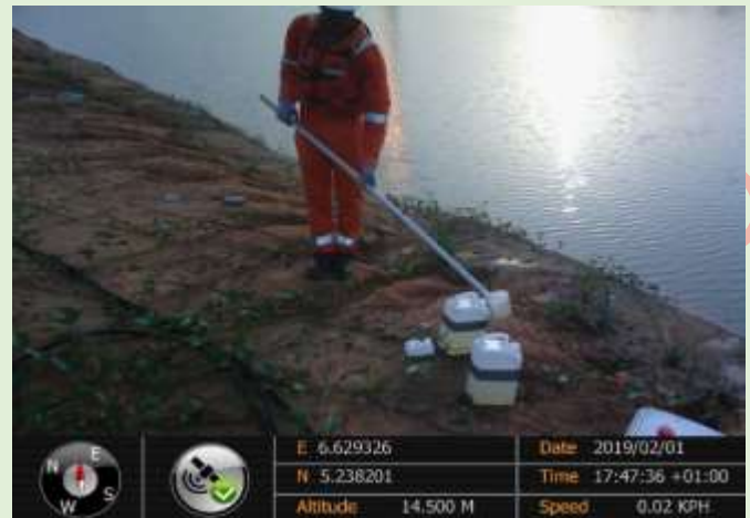
Plate 5: Surface Water Collection from Flare Pit at OB93/5B
